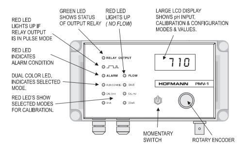
FIG 2 LED's show different mode of operation
