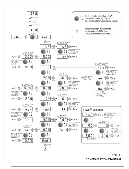
When dialing up numbers such as a setpoint, the encoder steps in single digits if turned slowly. To change large numbers quickly rotate the encoder in a "flicking" manner.
