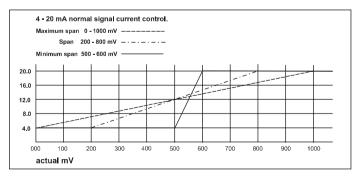
FIG 8 4-20mA normal Signal current control.
