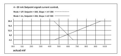
FIG 9 4-20mA Setpoint Signal current control.
